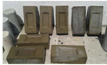
Fig. 6 Efflorescence Tested Specimens
